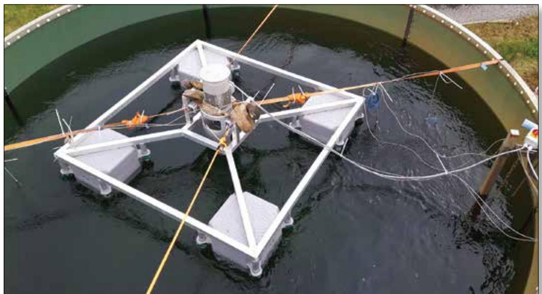
A new design of surface aerator being trialled (R. Cooney)
