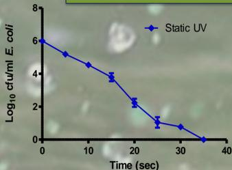
Figure 4. The effect of static UV light on *E. coli* (D Value = 4.80)
