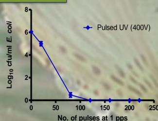
Figure 6. The effect of pulsed UV light on *E. coli* (D Value = 17.40)
