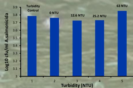
Figure 8. The effect of turbidity on PUV inactivation of *Aeromonas salmonicida* at 400V & 20 pulses (1pps).
