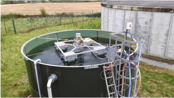
**Picture 2:** The recent testing of a surface aeration unit which uses the principal of mechanical shearing to aerate water with microbubbles in the 50-500µm range.
